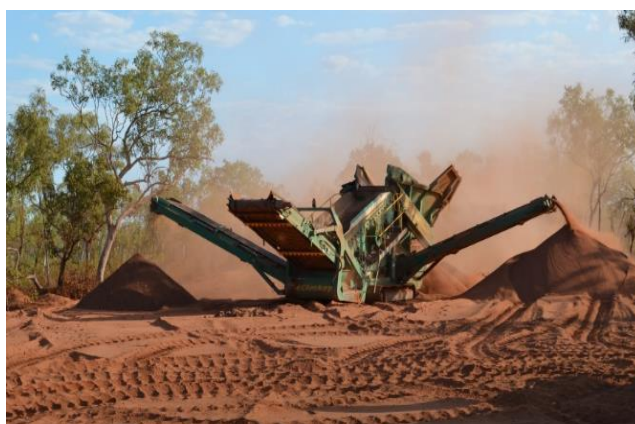
Figure 24: Mobile Screening Plant
