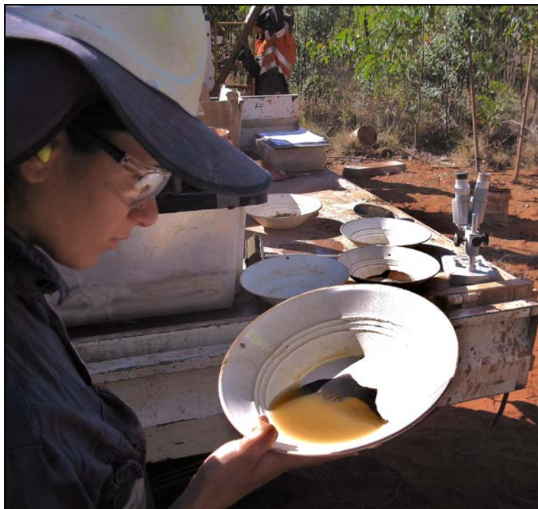
Panned heavy mineral concentrate from drilling at Thunderbird
