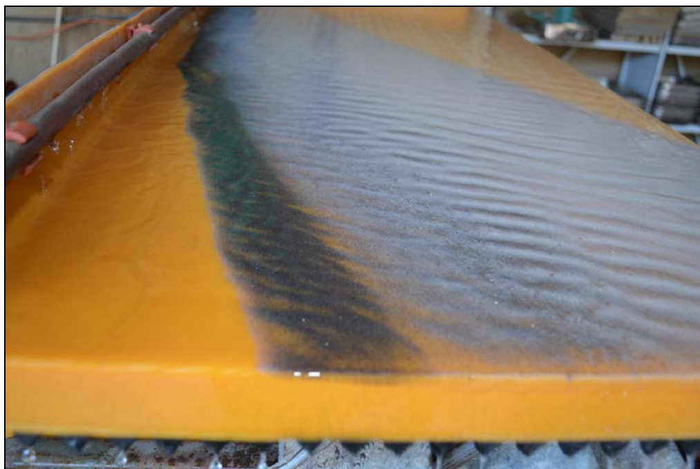
Wet table separation of heavy mineral from McCalls
