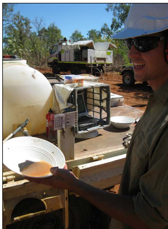
Panning heavy mineral from drill samples
