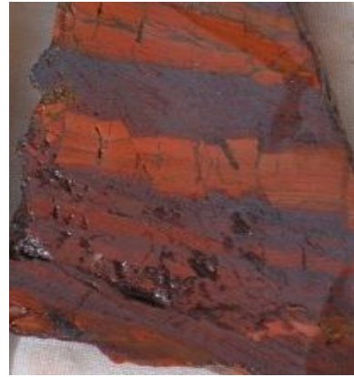
Figure 4: Banded Hematite/magnetite-jaspillite mineralisation
