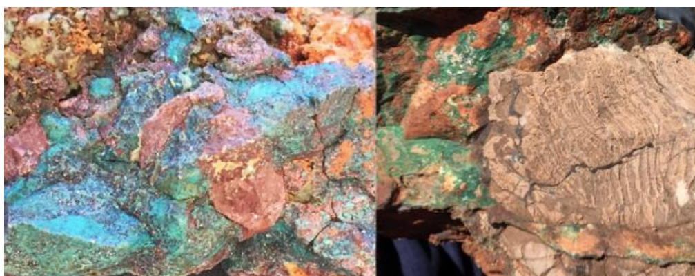
Figure 13: Western Star prospect - copper breccia (left), copper vein stock work in stromatolitic dolomite (right).
