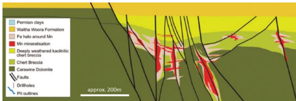
Figure 12: Reconstructed cross-section illustrating the geological setting and alteration of hydrothermal dolomite-replacement manganese mineralisation associated with pre-compression growth faults at the Greensnake deposit, Woodie Woodie Mine (after Jones, 2011). 29
