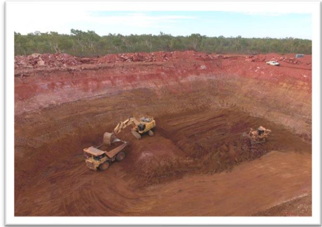
Figure 5: Ore mining by dozer push to fixed excavator location
