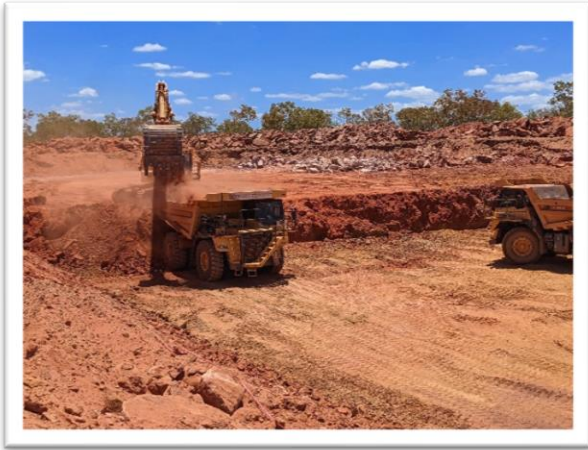
Figure 4: Waste mining by excavator and truck
