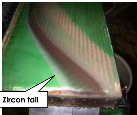
Cleaner stage gravity separation of HM on bulk sample from the Argo prospect. Source: Combined Annual Report (C96/2003 Mt Jowlaenga) for the Period 21 July 2007 to 20 July 2008 Rio Tinto Exploration Pty Ltd.
