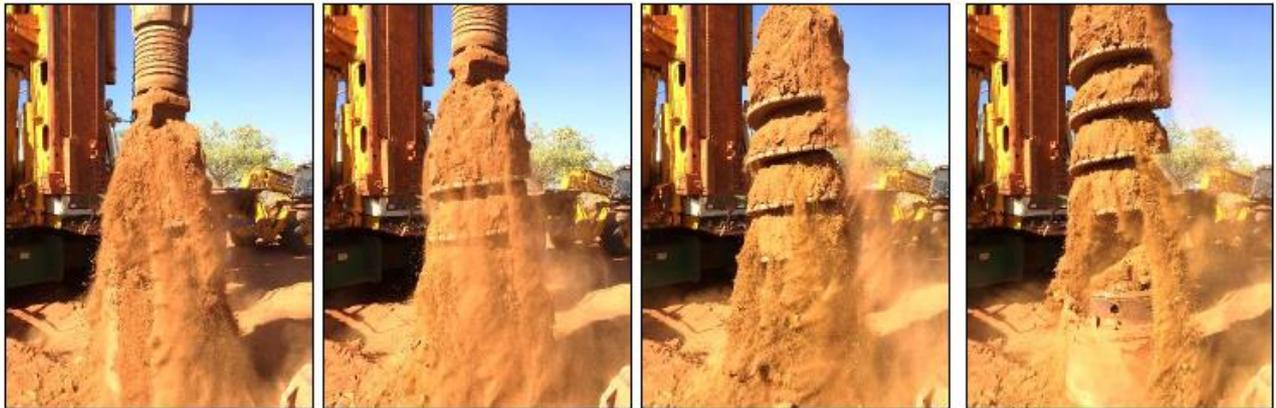
Figure 11: Sequence (from L-R) of Shallow Mineralisation Being Lifted from Bauer Hole THBA005, August 2015.
