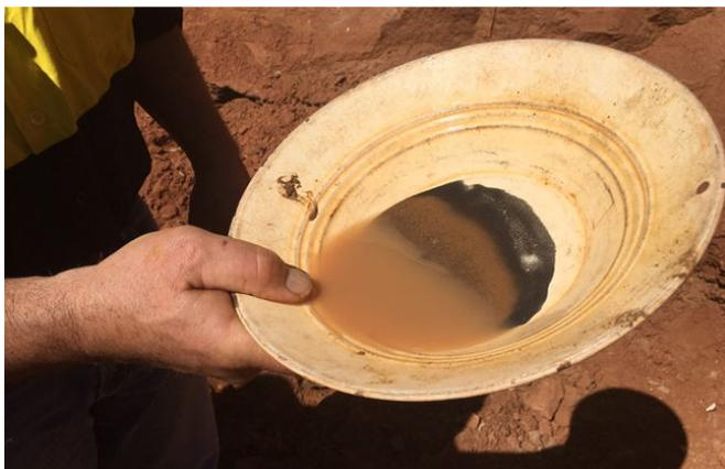
Above: Demonstrating how easy it is to separate the heavy minerals with simple panning.
