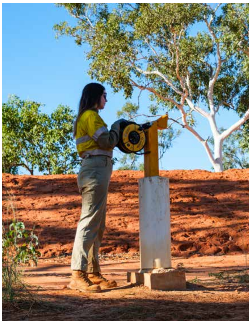
Figure 2: Groundwater monitoring being carried out by an Environmental Advisor
