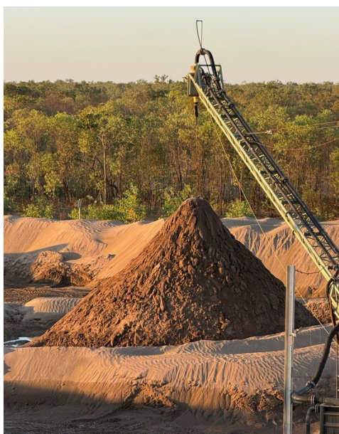
Zircon concentrate produced at around 20tph.
